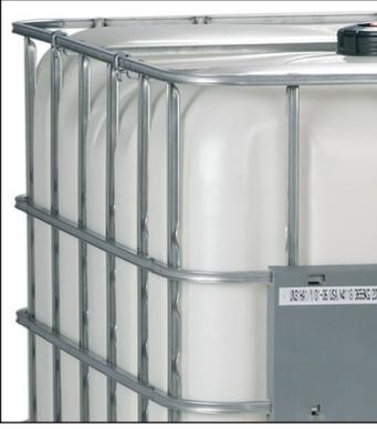
Offering the highest quality in space-saving bulk containers, this IBC is designed for multi-trip, hazardous and non-hazardous lading applications. It meets UN Standard 31HA1 for liquids in Packing Groups II and III with specific gravities up to 1.9.
